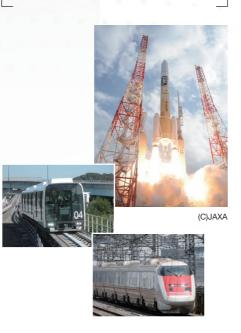
Rocket engine fuel pump displacement and vibration sensor Magnetic levitation control sensor for linear motor car Electric track general test vehicle rail displacement sensor
