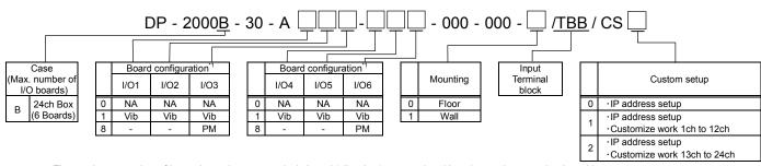
\*1 The maximum number of input channels on an analysis board (vibration/process signal input) or a phase marker board is 4
