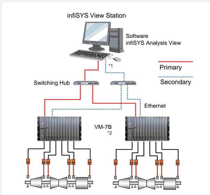
\*1 A LAN card must be added on the infiSYS View Station for secondary communication.
