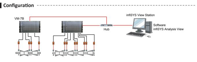
Waveform data can be collected at a minimum interval of 1 sec
