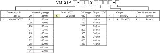
Note) • Standard specifications, when measuring range and full range of input LVDT are the same.
