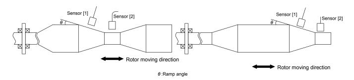
Note) The Above figure is typical example of attachment.
